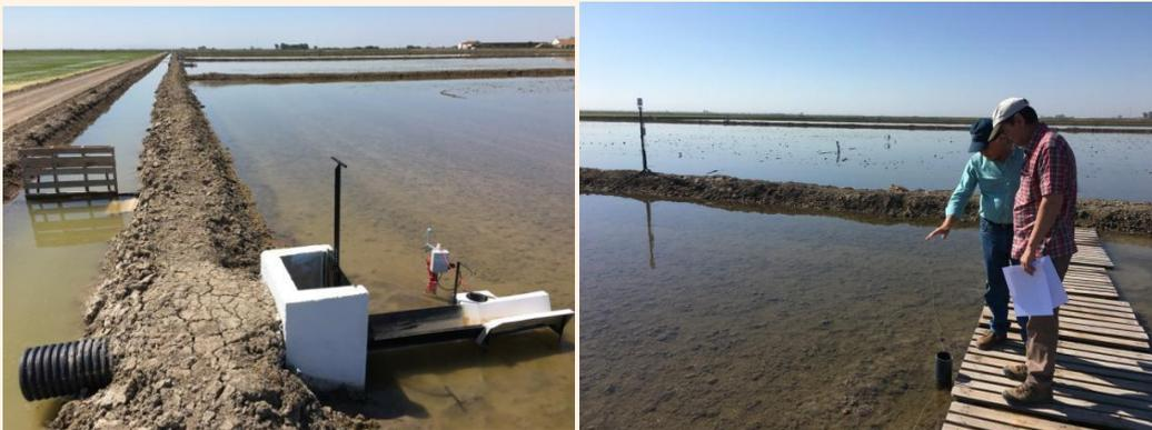
(Photo: *Experimentation plot, showing the sensors and systems to quantify water use + Electrical Conductivity in water inlet (left). Piezometers for visual inspection of water depth during the drying periods (right). Spain. Oryzonte Technical and Financial Report, 2018.*)
